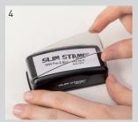
Select right colour of MaxLight Let ink soak in and put index card and cover lens back in place. Wait 45-60 minutes for ink to migrate and test stamp. Repeat steps if necessary.
